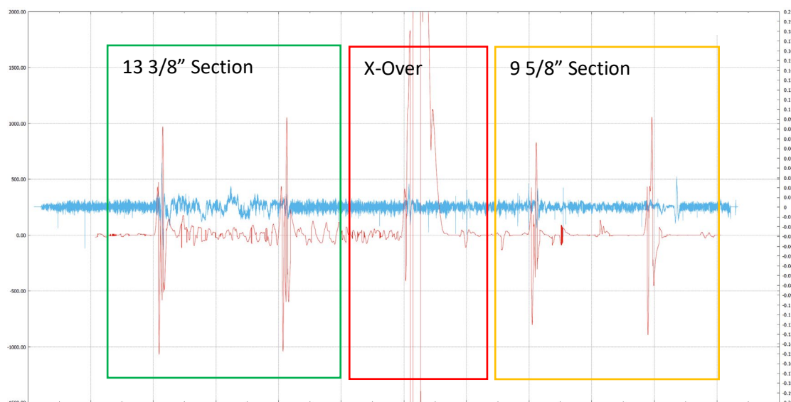
13 3/8 and 9 5/8" centralized data (CCL is lifted ~1.5" from casing) – 5 foot/min Red graph – left Y axis - NSE active CCL Blue graph – right Y axis – Standard industry CCL
