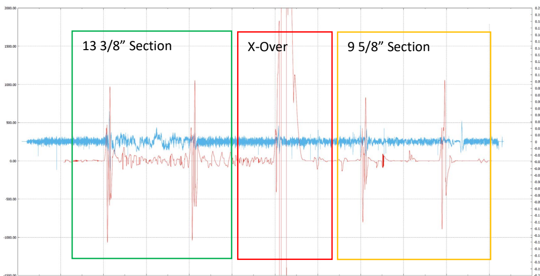
13 3/8 and 9 5/8" centralized data (CCL is lifted ~1.5" from casing) – 5 foot/min Red graph – left Y axis - NSE active CCL Blue graph – right Y axis – Standard industry CCL
