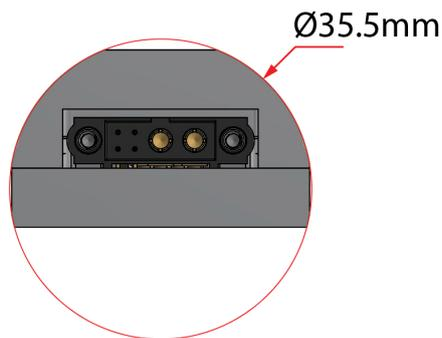
Figure 4 Unit inside ID=35.5mm
