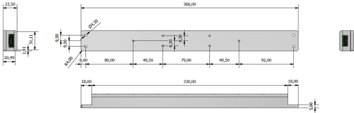
Figure 1 Mechanical dimensions
