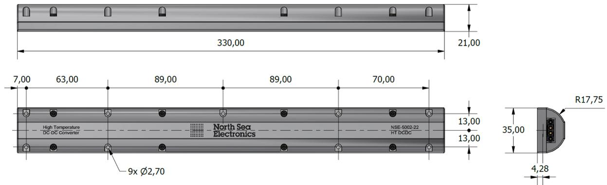
Figure 3 Mechanical dimensions
