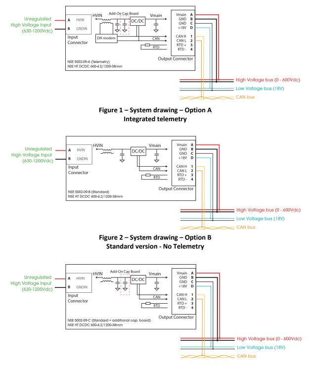
Figure 3 – System drawing – Option C Standard version with additional input capacitance Doc. no: -E
