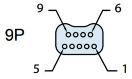
Illustration show face view of connector on the DL100 board (Looking in to the connector). Datasheet
