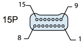
Illustration show face view of connector on the DL100 board (Looking in to the connector). Product no: NSE-5003-04
