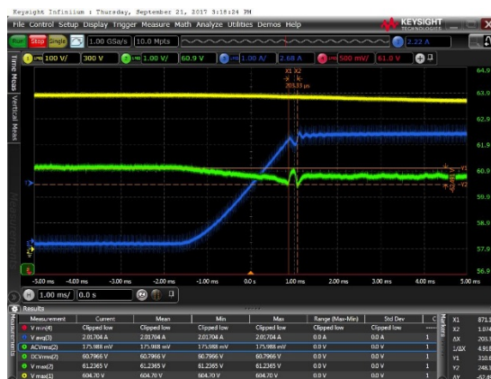
Figure 6. Step response with 600V input, 0 – 4.0A load. 1V/div, 1A/div, 1ms/div Result: 620mV drop
