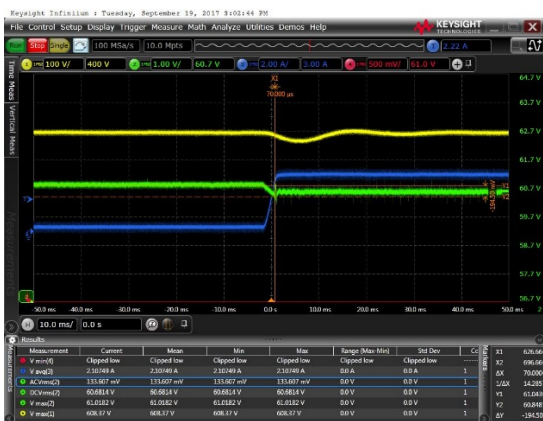
Figure 5. Step response with 600V input, 0 – 4.0A load. 1V/div, 2A/div, 10ms/div Result: 190mV drop
