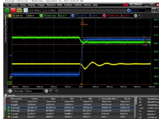
Figure 4. Step response with 100V input, 0 – 4.0 load. 500mV/div, 1A/div, 1ms/div Result: 440mV drop
