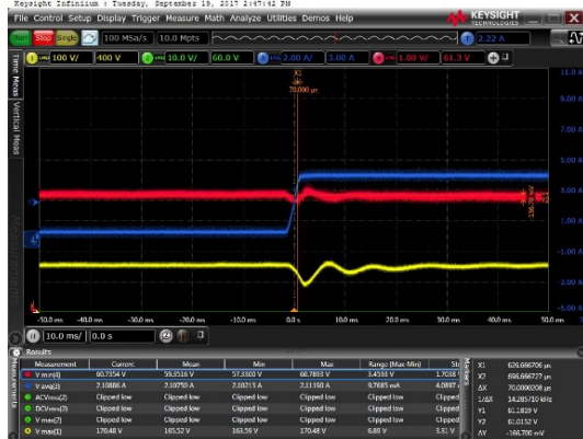
Figure 3. Step response with 100V input, 0 – 4.0 load. 1V/div, 2A/div, 500us/div Result: 170mV drop
