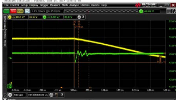
Figure 1 – Step response with 200V input, 0 – 4.2A load. 1V/div, 500us/div
