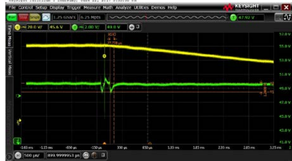
Figure 3 – Step response with 200V input, 0 – 4.2A load. 1V/div, 500us/div
