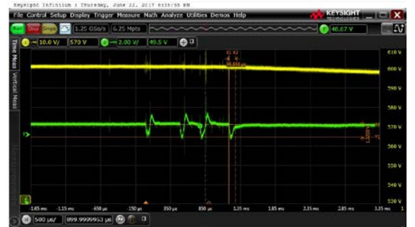
Figure 4 – Step response with 600V input, 0 – 4.2A load. 1V/div, 500us/div
