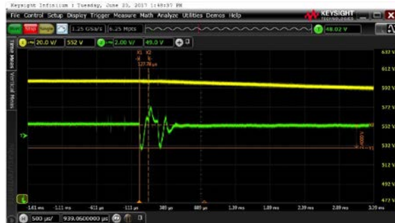
Figure 2– Step response with 600V input, 0 – 4.2A load. 1V/div, 500us/div
