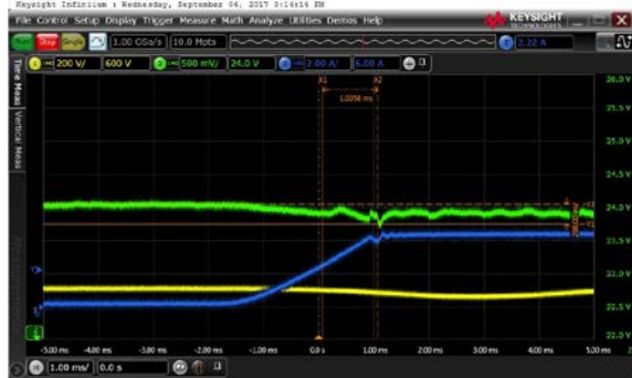
Figure 1 – Step response with 100V input, 0 – 4.0 load. 500mV/div, 2A/div, 500us/div Result: 1140mV drop
