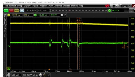
Figure 4 – Step response with 600V input, 0 – 4.2A load. 1V/div, 500µs/div
