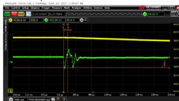
Figure 2– Step response with 600V input, 0 – 4.2A load. 1V/div, 500µs/div
