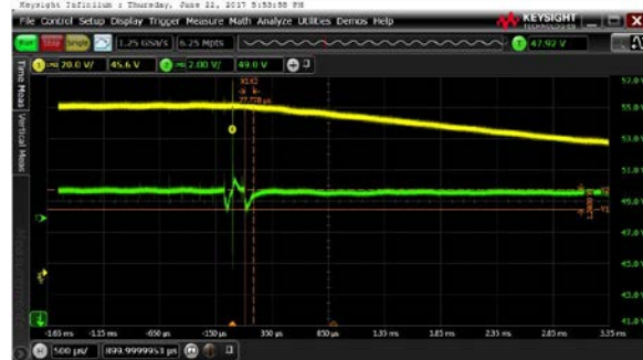
Figure 3 – Step response with 200V input, 0 – 4.2A load. 1V/div, 500µs/div
