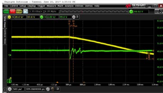
Figure 1 – Step response with 200V input, 0 – 4.2A load. 1V/div, 500µs/div
